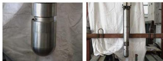
Figure 3. A) Test weight, B-End part of the weight
