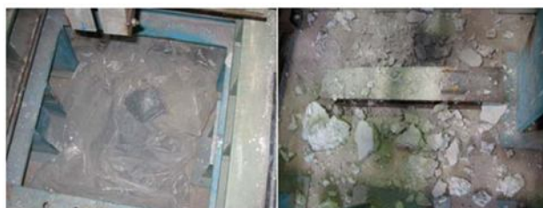
Figure 9. debris after A) the second impact on RC100 panel, B) the 17 th impact on ECC75
