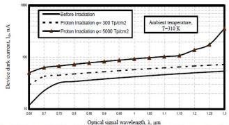
Fig. 10. Variations of the device dark current against optical signal wavelength at the assumed set of parameters.
