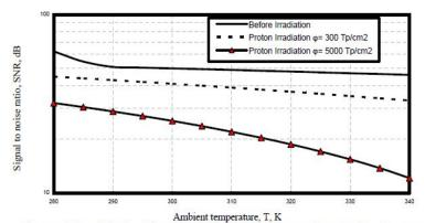
Fig. 7. Variations of signal to noise ratio against ambient temperature at the assumed set of parameters.
