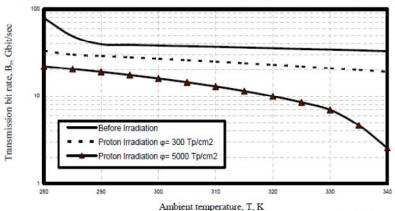
Fig. 6. Variations of transmission bit rate against ambient temperature at the assumed set of parameters.
