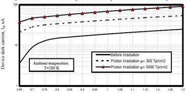
Optical signal wavelength,  $\lambda$ ,  $\mu m$ Fig. 9. Variations of the device dark current against optical signal wavelength at the assumed set of parameters.
