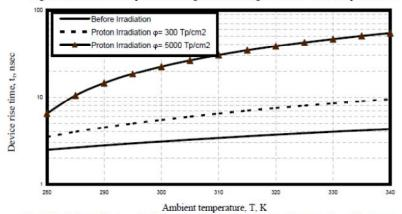
Fig. 5. Variations of device rise time versus ambient temperature at the assumed set of parameters.
