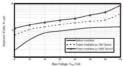
Fig. 4. Variations of the depletion width against bias voltage at the assumed set of parameters.
